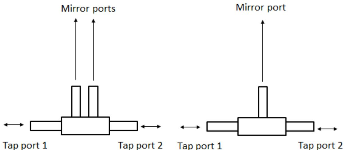
Figure 1, Network taps with one or two monitoring port
