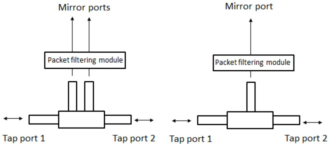
Figure 2, Network taps with packet filtering
