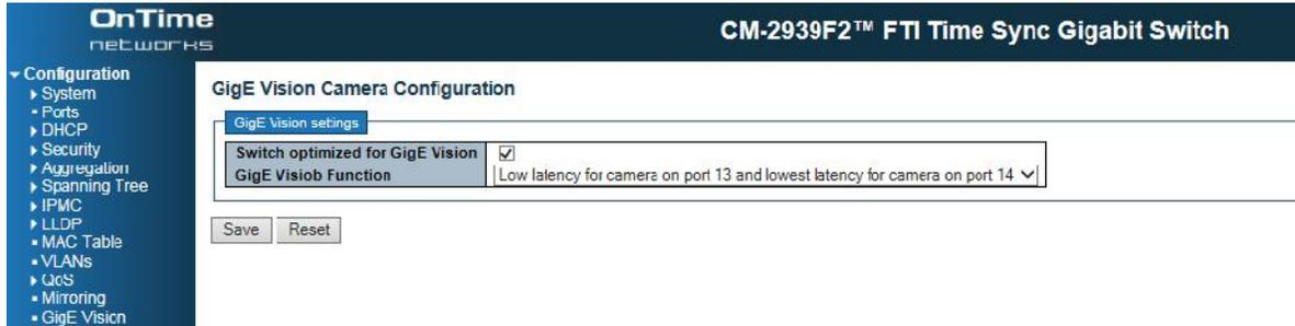
**Figure 5, GigE Vision switch setup for the switch with the two low latency sensitive cameras connected**
