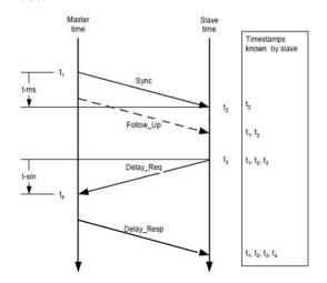
Figure 1, 1-step vs- 2-step clock
