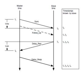
Figure 3, 1-step vs- 2-step clock
