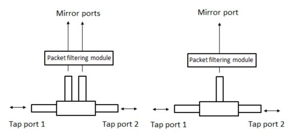
Figure 2, Network taps with packet filtering
