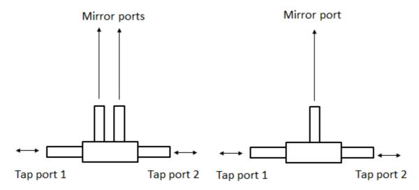
Figure 1, Network taps with one or two monitoring port
